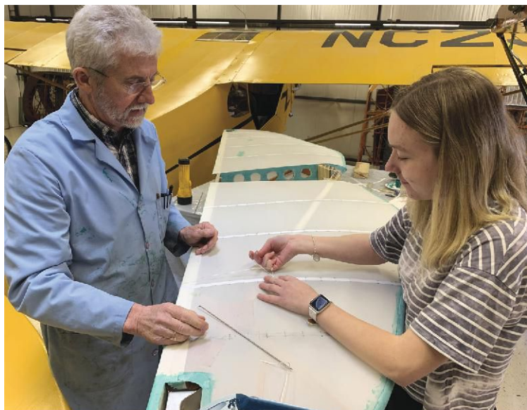
Perhaps one of the most psychologically difficult parts of restoring a classic biplane is covering the beautiful woodwork with fabric. But, that's what transforms it from sculpture to airplane.
